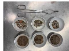
Fig. 6: Z1-Z6 soil samples first wet sieving and then dried
